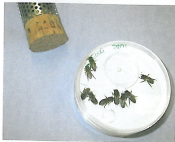
Figure 1. Laboratory testing of pesticide toxicity. Pesticides are applied in selected doses for different periods of exposure. The number of deaths at each dose and the duration of exposure are recorded for comparative analyses.
