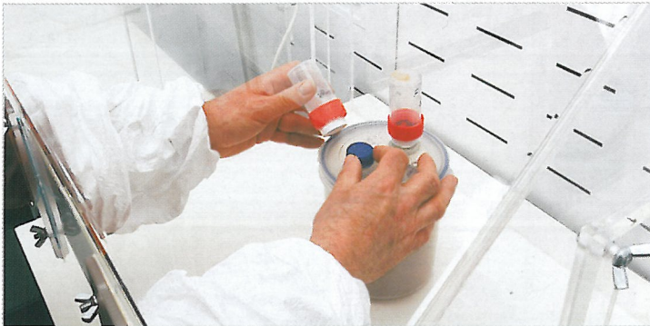
Figure 7. A scientist at work in the CE room, showing arms inserted into the Perspex culture cage through integral sleeves. Note also the inverted collection cylinders attached to the top of the culture box
